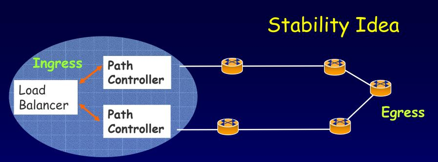
Per-path controller works at a faster timescale than load balancer  $\rightarrow$  Can decouple components  $\rightarrow$  Stabilize separately
