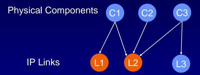
When {L1,L2} fail, it is not clear which components have failed: either {C1} or {C1, C2}
