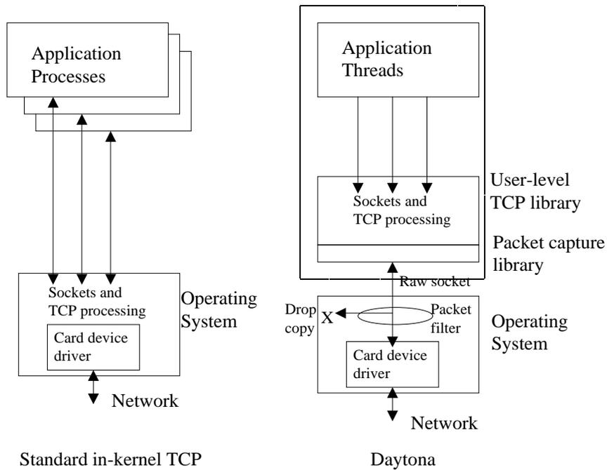
**Figure 1.** *The high-level design of Daytona compared to the stanrard in-kernel TCP stack.*
