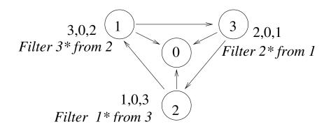
Figure 6-6: This routing system is stable without filtering but unstable under filtering. The figure shows a routing system with next-hop rankings and filtering that is equivalent to the unstable routing system with the rankings over paths shown in Figure 6-1.
