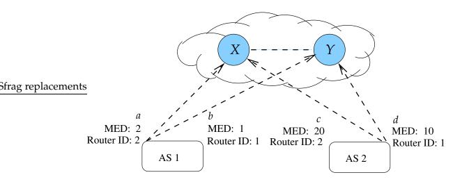
Figure 5-7: Interaction between MED and router ID in the BGP route selection process. *X* and *Y* are routers, each with direct eBGP sessions to ASes 1 and 2. *a*, *b*, *c*, and *d* are routes learned via eBGP.
