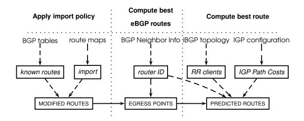
Figure 5-16: Data flow in the prototype. Fonts specify row inputs, *input tables*, and DERIVED TABLES. In practice, operators might collect raw inputs once a day.
