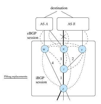
Figure 5-1: Network with three egress routers connecting to two neighboring ASes: Solid lines correspond to physical links (internal links are annotated with IGP link weights) and dashed lines correspond to BGP sessions. Thick lines illustrate the shortest path from one router to its closest egress point for reaching the destination.
