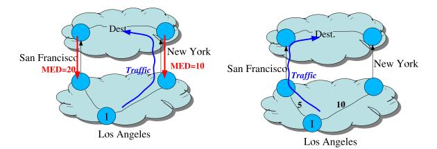
Figure 2-2: A neighboring AS can advertise routes to a destination with different MED values at different locations to control the exit point that routers in a neighboring AS uses to send traffic for that destination. When *I* learns both routes, it will select the route learned via the router in New York (and, thus, it will send traffic that way).
