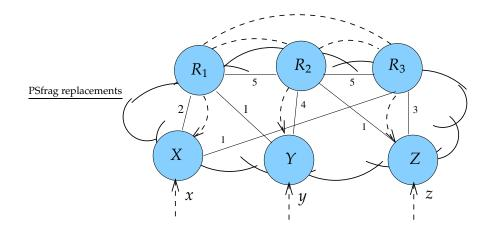
Figure 3-14: The interaction of IGP and iBGP can cause a violation of egress determinism that induces a safety violation. This figure shows the instantiation of Figure 3-13 in BGP. Previous work has also observed that violations of this type could occur [61] but did not observe that these could be constructed in general by composing egress determinism violations.
