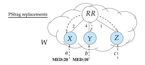
Figure 5-6: When an AS's iBGP topology uses route reflectors and MED, a router may not always select a route in  $\gamma(E)$ .
