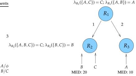
Figure 3-10: Instantiation of Figure 3-9 in a BGP configuration. Router 1 is a route reflector with two clients,  $R_2$  and  $R_3$ . Costs on edges are IGP path costs. Router  $R_2$  prefers route *B* over route *C* due to a tiebreak.
