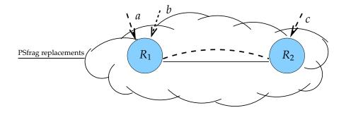
Figure 5-2: Route prediction requires resolving circular dependencies. Determining the route that  $R_2$  ultimately selects (*i.e.*, *a*, *b*, or *c*) first requires determining whether  $R_1$  selects route *a* or *b*. Ultimately,  $R_1$ 's selected route could depend on whether it learns route *c* from  $R_2$ , which requires revisiting  $R_1$ .
