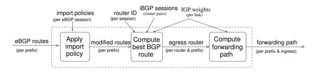
Figure 5-3: Our algorithms decompose network-wide BGP route selection into three independent stages. The algorithms take as input the eBGP-learned routes from neighboring ASes, the router IDs of each BGP session, and the routing configurations from all of the routers in the AS, which provide information about the IGP topology, the iBGP topology, and the import policies (*i.e.*, rankings) of each router.
