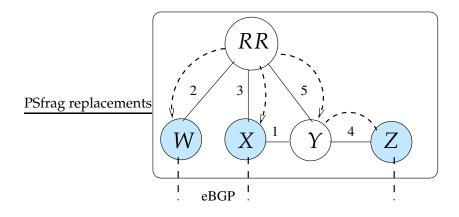
Figure 5-12: When an AS's iBGP topology uses route reflectors, a router may not always discover the route corresponding to its closest egress router.
