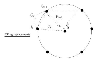
Figure 6-9: Illustration of a dispute wheel. Dotted lines show preferred (indirect) paths to the destination. The nodes  $i_1, \ldots, i_m$  are pivots.
