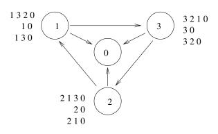
Figure 6-10: A routing system that is safe for any choice of filters.
