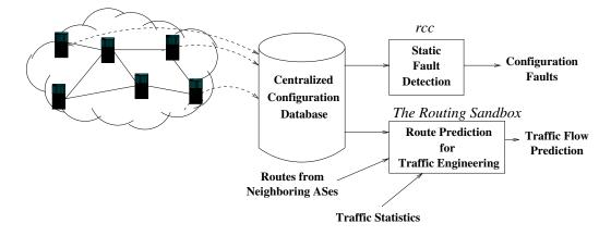
Figure 1-6: Workflow for fault detection and route prediction tasks described in this dissertation. Both fault detection and route prediction tasks rely on *offline* analysis of the distributed router configurations, which are first collected into a centralized database.
