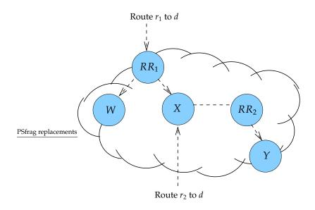
Figure 4-4: In this iBGP configuration, route  $r_2$  will be distributed to all the routers in the AS, but  $r_1$  will not.  $RR_2$  and Y will not learn of  $r_1$ , leading to a network partition that won't be resolved unless another route to the destination appears from elsewhere in the AS.
