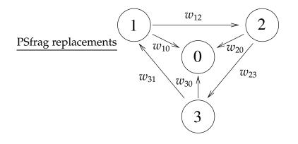
Figure 6-7: Routing system with edge weight-based rankings.
