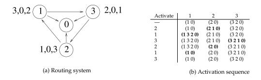
Figure 6-5: Next-hop rankings are not safe in this routing system. AS 1 prefers all paths through AS 3 over the direct path to the destination 0 (with ties broken deterministically) and prefers the direct path over all paths through AS 2. Similarly, AS 3 prefers all paths via AS 2, and so forth.
