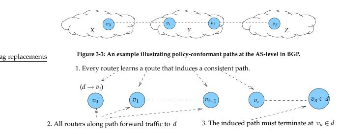
Figure 3-4: The conditions of route validity. A route is valid if it induces a consistent, policy-conformant path at every node along the path from  $v_0$  to some  $v_i \in d$ .
