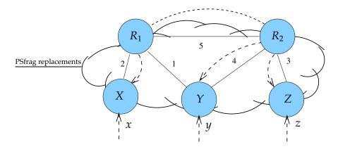
Figure 3-12: The interaction of IGP and iBGP can cause a violation of egress determinism.  $\lambda_{R_1}$  is equal to either *x* or *y* depending on whether  $z \in E_d$ .
