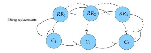
Figure 3-7: A simple iBGP topology that violates path visibility. Routes learned via eBGP at  $RR_1$  or  $C_1$  will not be propagated to  $RR_3$  or  $C_3$  (and vice versa).
