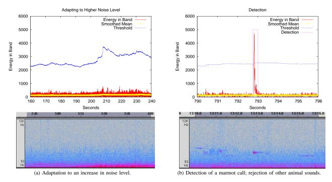
Fig. 6. Behavior of the CFAR-based marmot alarm call detector.
