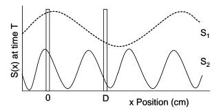
Fig. 3. The spatial aliasing problem. Sensors at position 0 and D observe the same phase offset for signals  $S_1$  and  $S_2$ . When measured phase offsets are used to deduce direction of arrival, ambiguities result for signals with  $\lambda < 2D$ .
