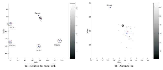
Fig. 17. Scatterplot of location estimates from wide deployment after removing node 108 and 106.  $\mu = (82.6, 14.2)$ , and  $\sigma = (1.4, 2.8)$  meters.
