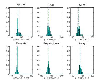
Fig. 11. Histograms of the maximum DOA estimates for the same data shown in figure 10, grouped by distance and grouped by source facing. Each plot shows mean  $\mu \pm$  the standard deviation and the median m.
