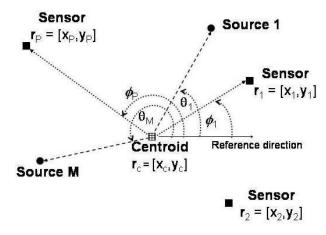
Fig. 7. Far-field notations for sources, sensors, and sensor array centroid
