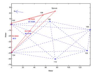
Fig. 14. Wide deployment comparison between node self-localization and GPS data. GPS data is denoted by round circles connected in a solid line.
